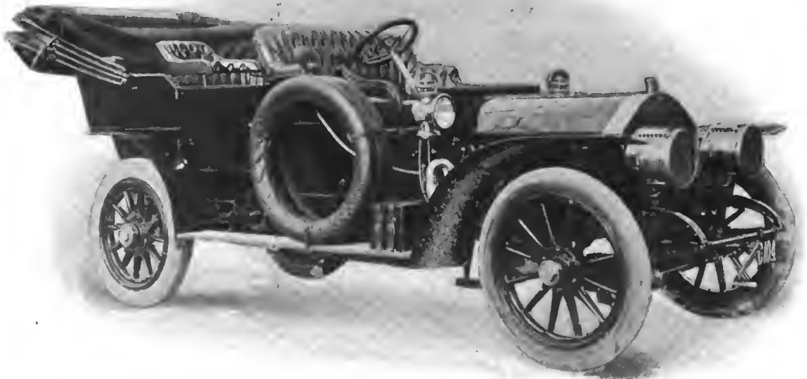
COLUMBIA GASOLINE-ELECTRIC TOURING CAR, 4 CYLINDERS, 48-H.P., PRICE $6,500. Electric Vehicle Co., Hartford, Conn.
